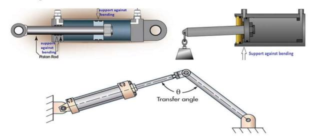
Cylinder is hinged at one position so it is free to move in its pin but due to high axial force of spring on pin and wear of pin, it will always creates some frictional resistance and restrict its rotation which is sufficient to create such type groove after running of a certain duration.
