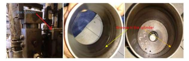
At bottom of the cylinder hydraulic pressure is around 8kg/cm2 and after crossing piston is pressure is 2kg/cm2 (line back pressure) connected to drain. P1-P2=6kg/cm2
